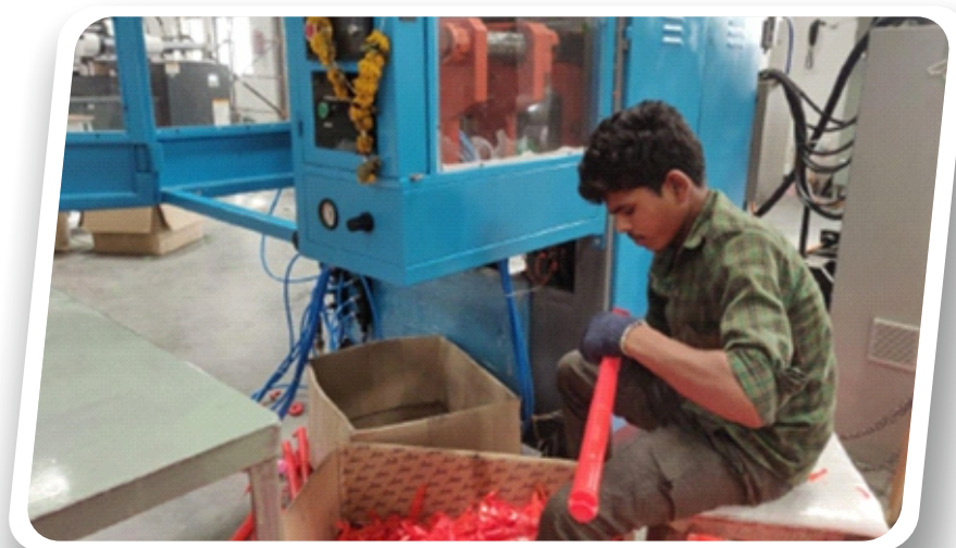
Injection Molding Machine- Milacron, USA (110MT to 550MT)
